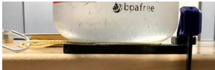
Figure 31: Calibrated Weight, Dyneema, NylonX Sample Stack
