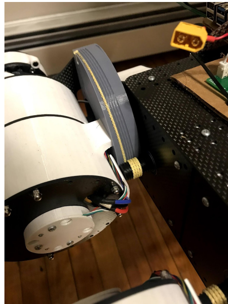
Figure 41: Final Capstan Prototype
