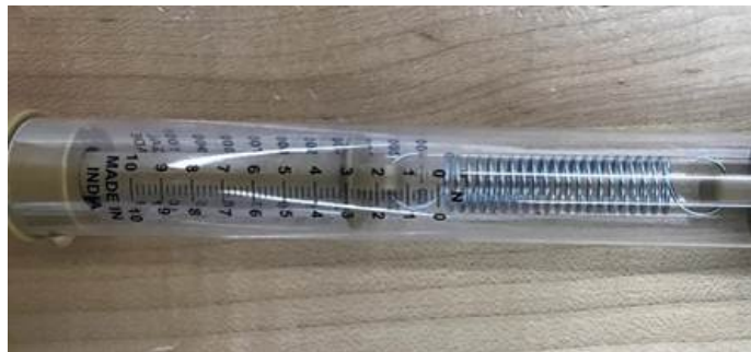
Figure 32: Force Gauge Reading when the Static Friction Force Was Broken
