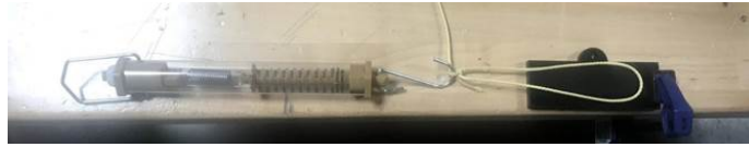
Figure 30: Full Dyneema NylonX Friction Test Setup
