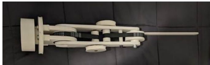
Figure 10: Partially Assembled First Version of Leg
